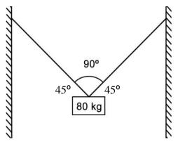
2. Find the tension in cables A and B if the mass of the sign is 80 kg?
